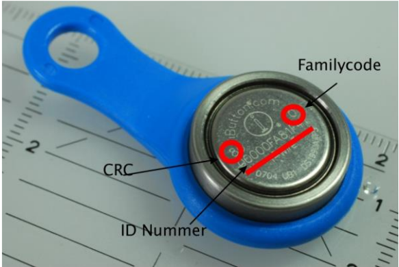
Figure 4: Meaning of lasered labeling of the key
