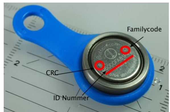
Figure 4: Meaning of lasered labeling of the key
