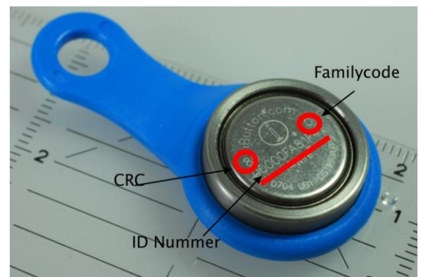
Figure 4: Meaning of lasered labeling of the key
