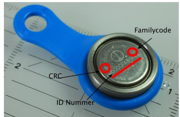
Figure 4: Meaning of lasered labeling of the key
