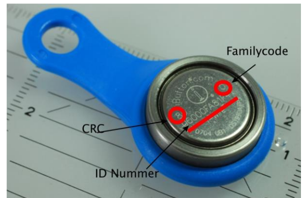
Figure 4: Meaning of lasered labeling of the key
