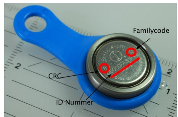
Figure 4: Meaning of lasered labeling of the key
