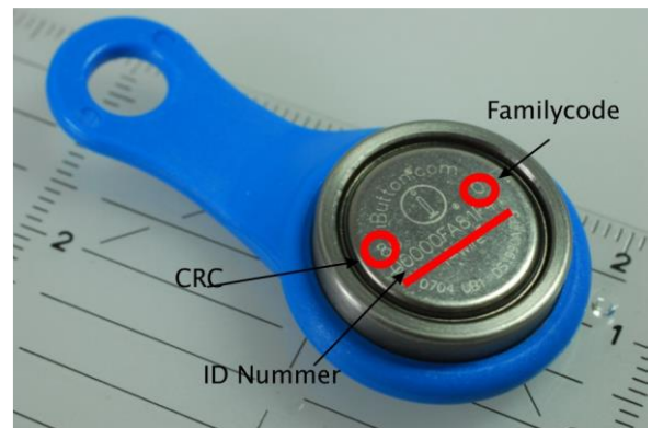
Figure 4: Meaning of lasered labeling of the key
